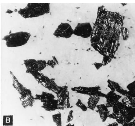
**Fig. 3.** Photomicrographs of particles found in samples submitted to the Arizona AMS laboratory by Dorn. (A) Type II grain found in a petroglyph sample (EK95-8). This grain is about 1 mm long. (B) Both type I and type II grains found in Dorn sample AA 2321. The typical size of type II grains shown is approximately 0.2 to 1.0 mm.
