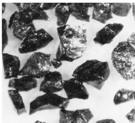
**Fig. 2.** Photomicrograph of typical type I particles separated from samples submitted to the Arizona AMS laboratory by Dorn. These particles were found in sample AA 2321. Note blocky, angular, surfaces with well-developed conchoidal (glassy) fracture. The typical size of grains shown in these photos is 0.2 to 0.6 mm.
